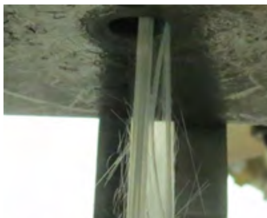
Figure 5. CeraFib 99 fiber roving fed into the inlet orifice, prepared for pulling across
