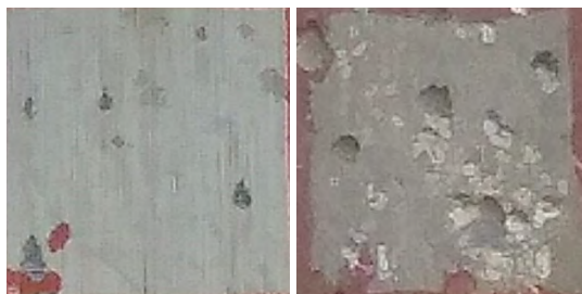
Figure 2. N. 2. samples: a) without heat treating, b) heat treated
