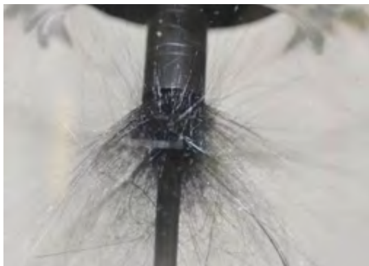
Figure 3. Fluffing of the carbon fiber tow at the entrance of the inlet orifice made of graphite
