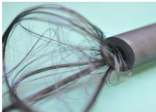
Figure 3. Fluffing of the carbon fiber tow at the entrance of the inlet orifice made of graphite
