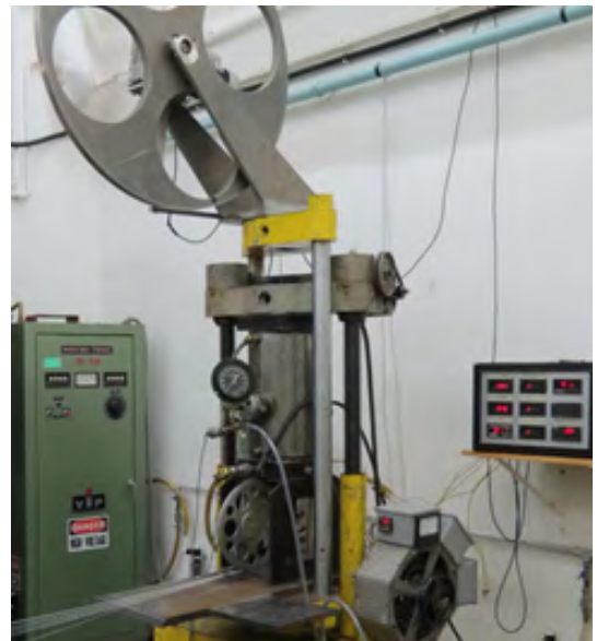
Figure 8. Pulling across the fiber roving of five tows in the Blücher process
