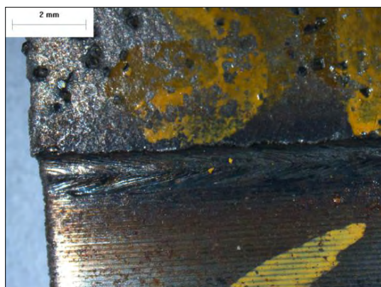
Figure 1. Stereo microscope recording of the laser welded seam from the crown side
