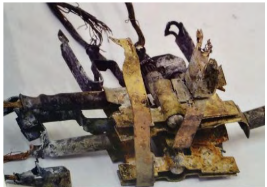
Figure 2. Galvanic corrosion affected damage
