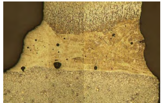
Figure 3. Optical microscope recording of the laser welded seam
