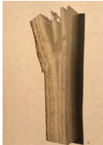
Figure 4. Picture of the sample after dynamic impact load [11]
