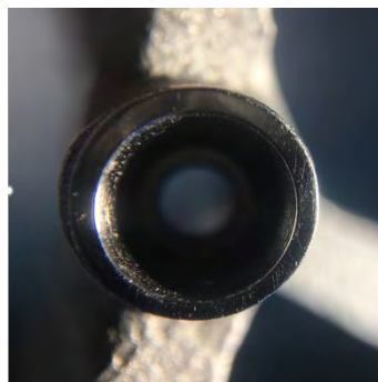
Figure 4. The implanted fitting surface after processing
