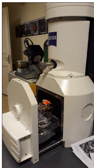
Figure 2. Placement of stent clamping and rotating prototype in the chamber of a Zeiss EVO MA 10 scanning electron microscope
