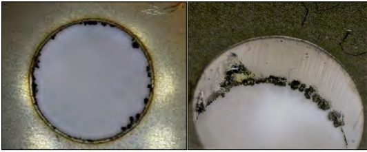
Figure 1. Adherent iron-oxide on the hole surface cut with CO 2 laser (∅ 6,2 hole)
