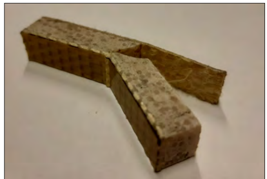
Figure 14. Aramid fiber weave and epoxy resin laminated test sample after test
