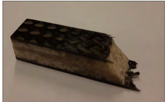
Figure 13. Carbon fiber weave and epoxy resin laminated test sample after test
