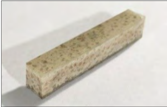
Figure 6. Glass fiber weave and epoxy resin laminated test sample
