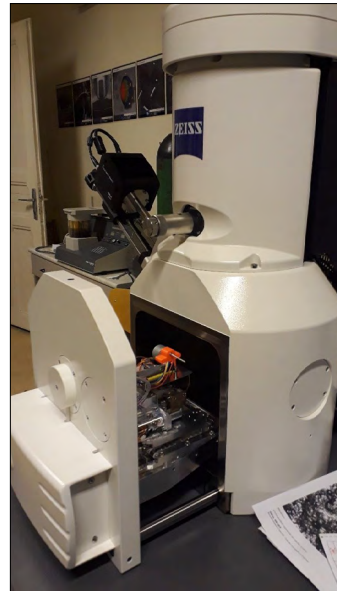
Figure 2. Placement of stent clamping and rotating prototype in the chamber of a Zeiss EVO MA 10 scanning electron microscope
