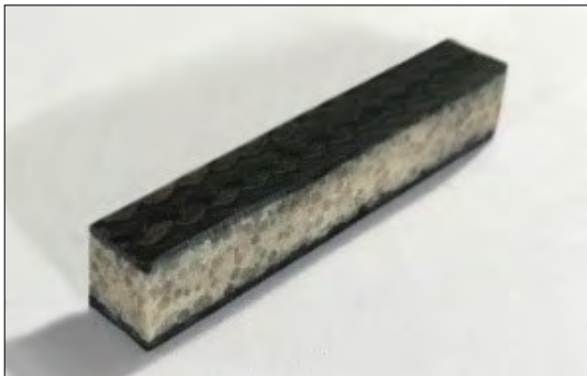
Figure 7. Carbon fiber weave and epoxy resin laminated test sample
