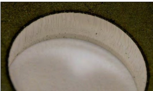
Figure 4. Hole made with Disk laser (∅ 13,6 hole)
