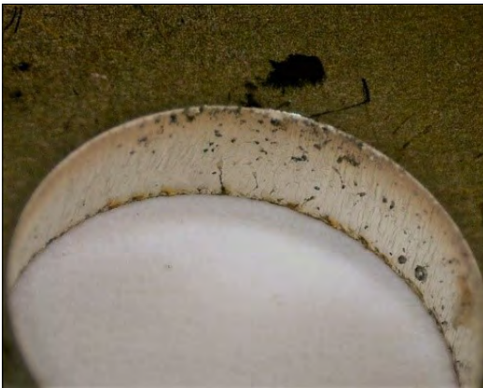
Figure 7. The cut made with disc laser, with changed focus distance from the centerline ( \varnothing 13,6 hole)
