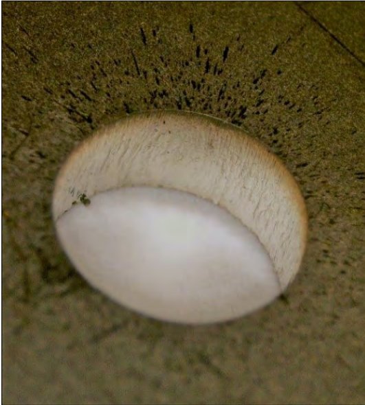
Figure 6. Spatter on the rim of the laser cut hole in the disc ( \varnothing 6,2 hole)
