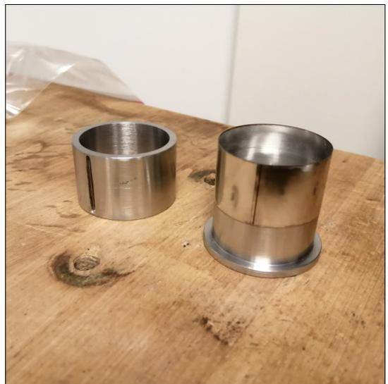
**Figure 5.** Successfully welded mantle with mantle welder fixture.
