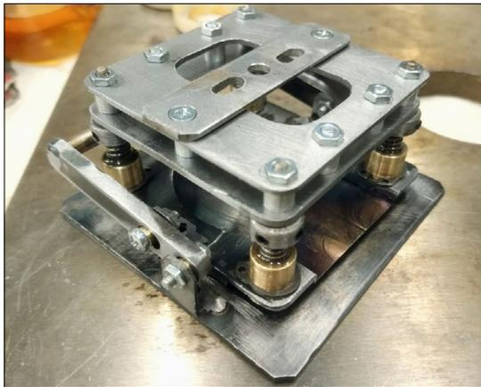
**Figure 5.** The assembled device without the PDMS cell.
