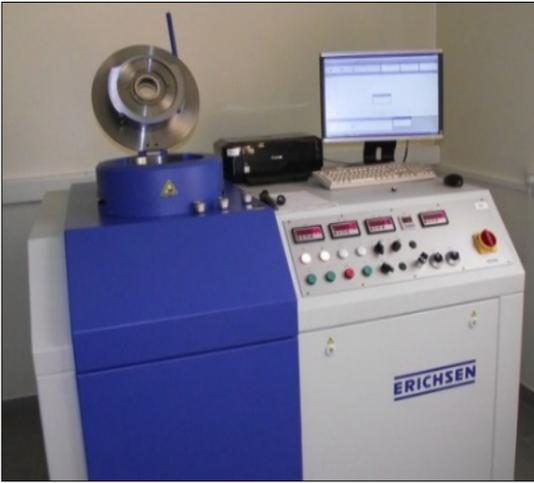
Figure 7. The applied universal sheet metal tester equipment.
