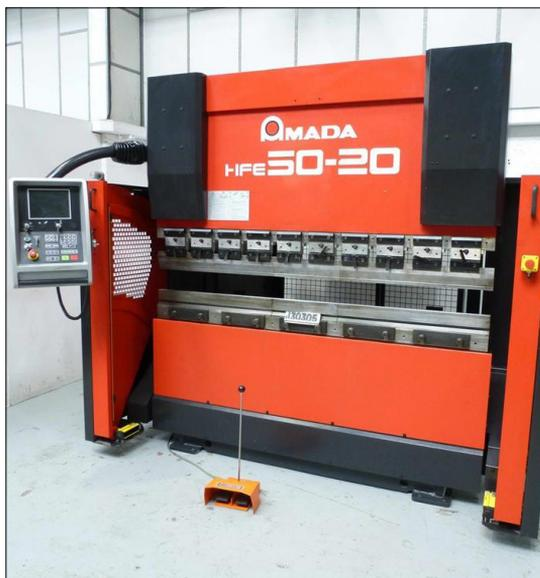
**Figure 2.** The applied Amada bending machine.
