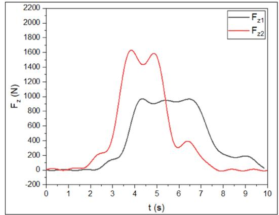
**Figure 7.** Cutting forces  $F_z$  measured in the Experiments 1-2. as a function of machining time.
