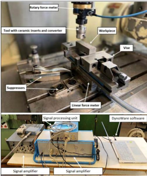
Figure 3. Experimental setup.
