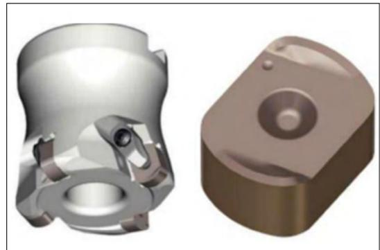
Figure 5. The cutting tool holder and insert used for the experiment.
