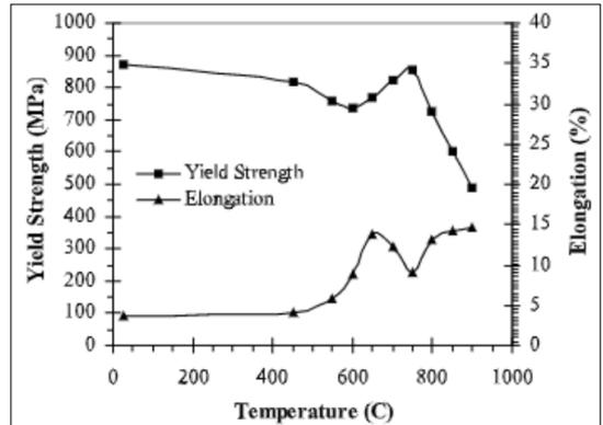
**Figure 2.** Temperature dependence of yield strength and elongation of GTD-111. [11]
