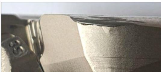
**Figure 6.** Damaged tool body.
