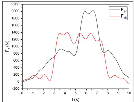
**Figure 9.** Cutting forces  $F_z$  measured in the Experiments 7-8. as a function of machining time.
