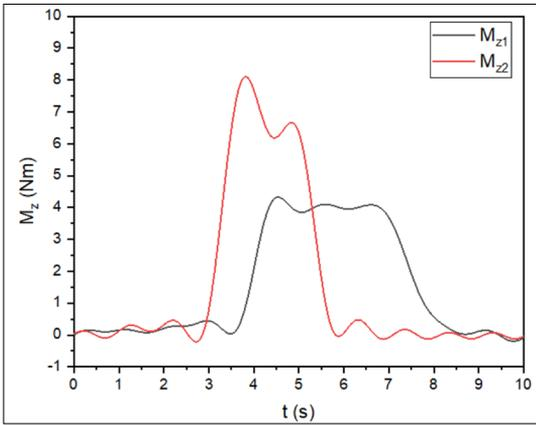
**Figure 10.** Cutting torques  $M_z$  measured in the Experiments 1-2. as a function of machining time.
