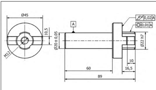
Figure 4. Drawing of the intermediate piece required to clamp the tool.
