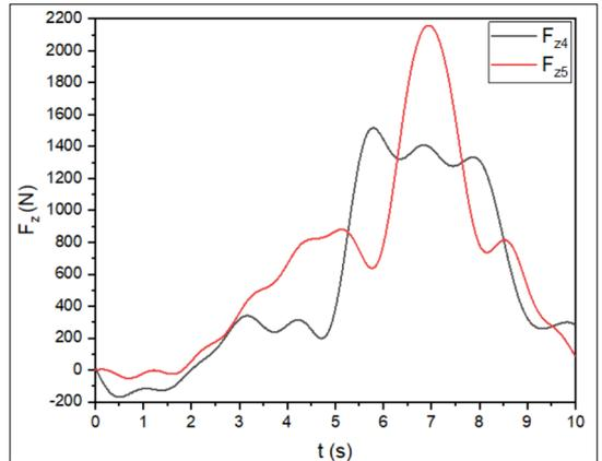
**Figure 8.** Cutting forces  $F_z$  measured in the Experiments 4-5. as a function of machining time.
