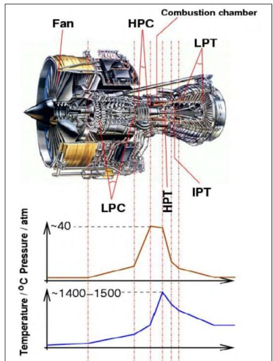
Figure 1. Gas turbine showing the different zones with temperature and pressure conditions [8]
