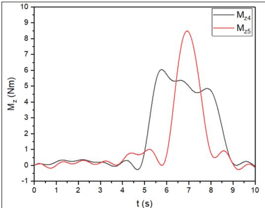
**Figure 11.** Cutting torques  $M_z$  measured in the Experiments 4-5. as a function of machining time.
