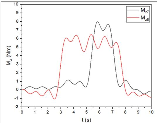
**Figure 12.** Cutting torques  $M_z$  measured in the Experiments 7-8. as a function of machining time.
