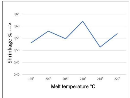
Figure 9. Effect of melt on shrinkage.
