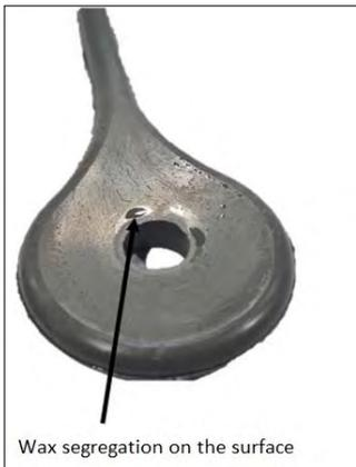
Figure 7. Wet product surface, possible wax separation.
