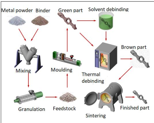
**Figure 1.** The process flowchart of metal injection moulding [3]
