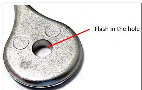
**Figure 4.** Burring of the test specimen's hole.
