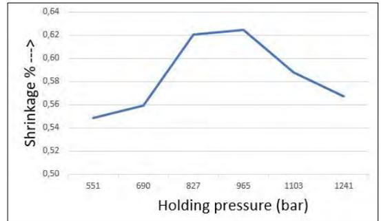
Figure 8. Effect of holding pressure on shrinkage.
