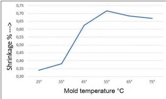
Figure 6. Effect of tool temperature on shrinkage.
