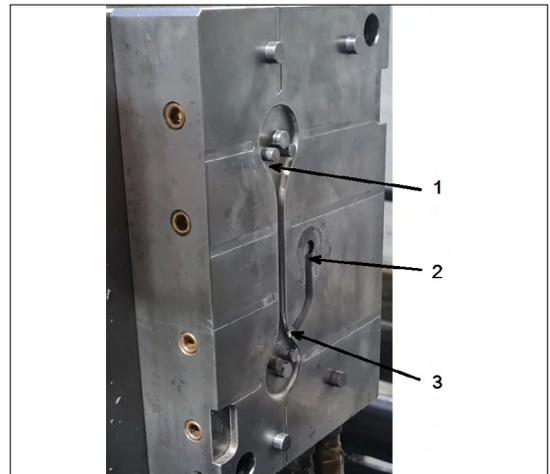
**Figure 2.** The tool used for the test. 1- Cavity, 2-Runner, 3-Gate
