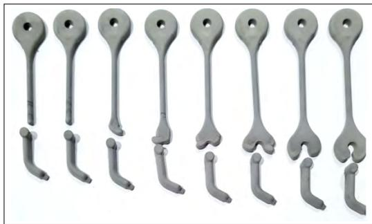
**Figure 3.** Fill sequence to define the switching point.
