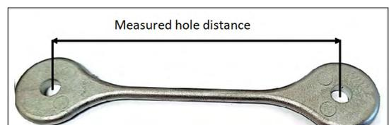
**Figure 5.** Measured value of linear shrinkage.
