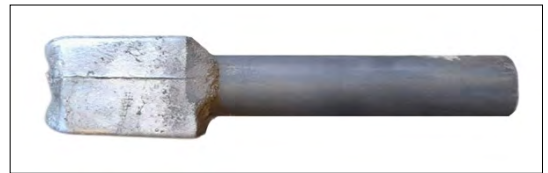
Figure 2. In-situ produced syntactic metal foam-filled steel tube, after cooling.
