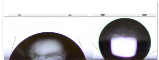
**Figure 1.** The most widely spread (left) and the least widely spread (right) drop during the measurements.
