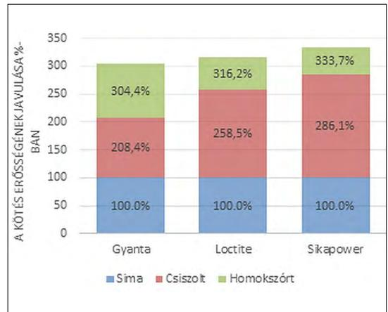
**Figure 3.** Effect of surface treatments compared to untreated surface.
