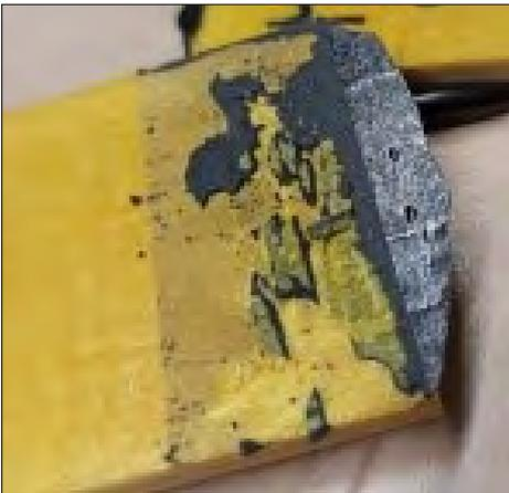
**Figure 2.** The partially peeled off adhesive bond on the sandblasted profile with Sikapower adhesive.
