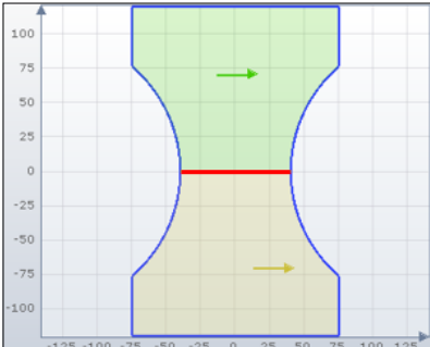
Fig. 6. Location of weld seam, type „B”
