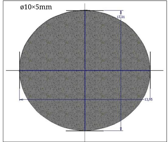
**Fig. 8.** The difference in diameter between the rolling direction and the perpendicular direction.
