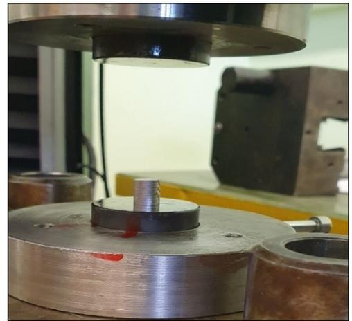
**Fig. 4.** Execution of the compression tests.
