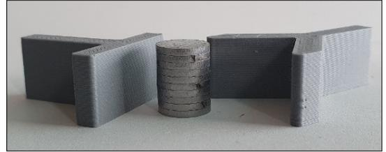
**Fig. 3.** Positioning unit and the stack made by it.
