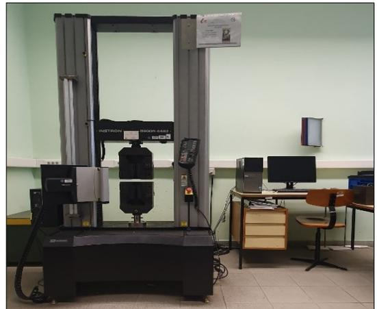
**Fig. 1.** Instron4482 electromechanical universal testing machine.
