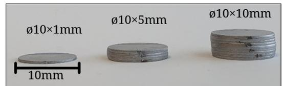
**Fig. 5.** The stacks after compression test.
