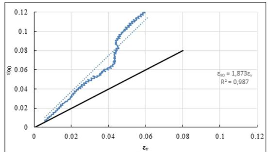
**Fig. 9.** Anisotropy (R) Value Determined from Tensile Testing.
