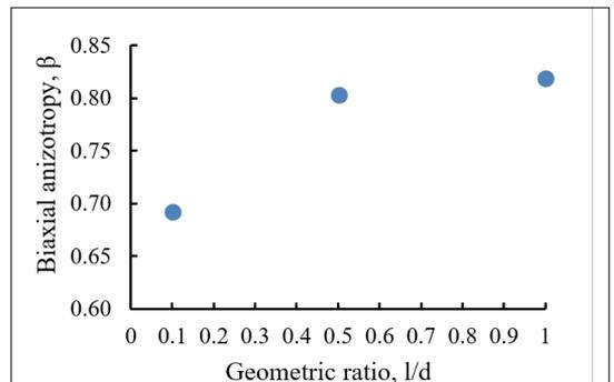
**Fig. 10.** The change in biaxial anisotropy (R) value as a function of the  $l/d$  ratio.
