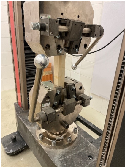
Fig. 12. Adhesion testing of resin applied on the sectional side of the wood.
