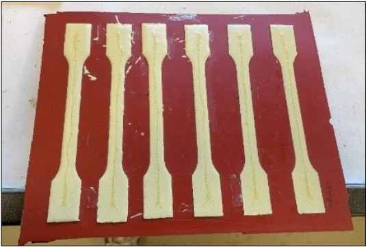
Fig. 2. Test specimens used to determine the tensile strength of the resin.
