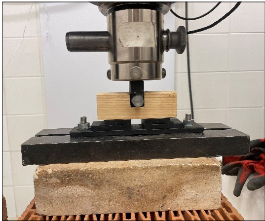
Fig. 19. Shear load test with weakening.
