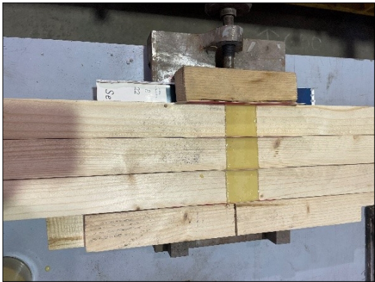
Fig. 25. Filling the weakened timber parts with epoxy resin.
