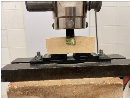
Fig. 21. Shear test specimens supplemented with resins.
