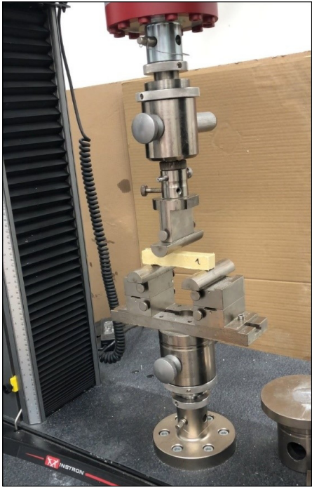
Fig. 8. Resin specimen tested for bending.
