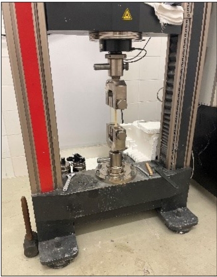
Fig. 3. Measurement of tensile strength of resin.
