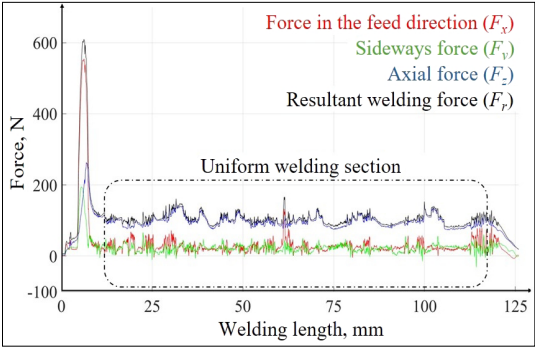
Fig. 4. Force components during welding.
