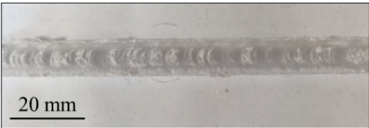
Fig. 8. A characteristic seam from a top view.
