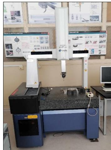
**Fig. 4.** Mitutoyo Crysta Plus M574 measuring machine.
