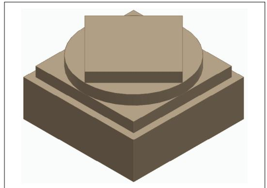
**Fig. 1.** NASA test (workpiece).
