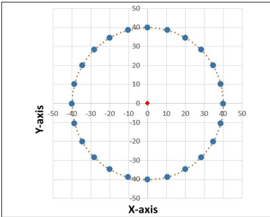
Fig. 6. OMM measurement of the round shape with 24 points.
