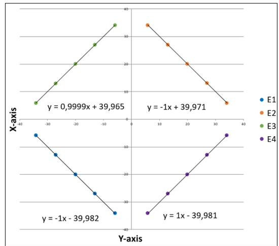
**Fig. 5.** OMM measurement result of a square rotated by 45°.
