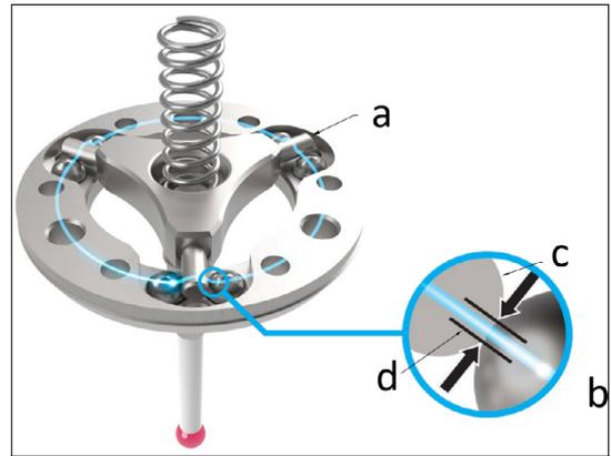
**Fig. 2.** Switch type probe operating principle. [5]
