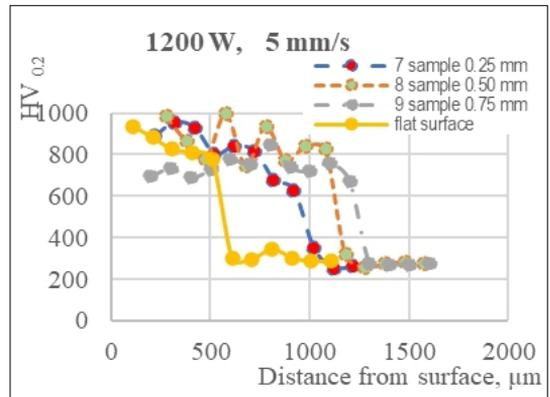
Fig. 9. Hardness plots as a function of distance from the surfaces in case of 240 W s/mm specific laser heat input.
