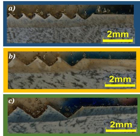
Fig. 8. Micrographs taken after heat treatment with 240 W s/mm specific laser heat input a) 0.25 mm depth grooves, sample nr. 7, b) 0.5 mm depth grooves, sample nr. 8 c) 0.75 mm depth grooves sample nr. 9.
