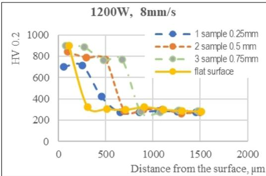
Fig. 4. Hardness as a function of depth in the case of 150 W s/mm specific laser heat input.
