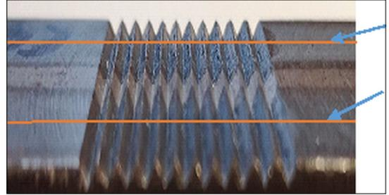
Fig. 2. The appearance of 0.75 mm deep milling grooves after heat treatment The arrows show the position of the metallographic samples cutting line.
