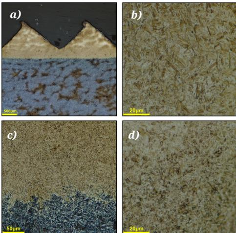
Fig. 5. Micrographs from hardened surface layer a) Microstructure of 0.75 deep milling grooved zone b) high resolutions micrographs martensitic microstructure near surface c) transition zone between surface layer and core of bar d) heat treated zone under grooves
