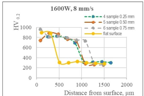
Fig. 7. Hardness versus depth curves for 200W s/mm specific laser heat input.
