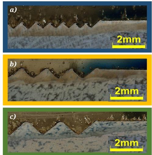
Fig. 6. Effect of laser hardening at 1600 W and 8 mm/s on grooved surfaces a) 0.25 mm grooves, sample nr. 4, b) 0.5 mm grooves, sample nr. 5, c) 0.75 mm grooves, sample nr. 6.
