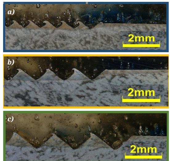
Fig. 3. Micrographs after heat treatment with 150 Ws/mm specific heat input a) sample nr. 1 b) sample nr. 2 c) sample nr. 2.
