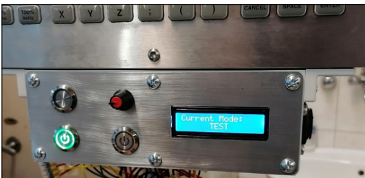
Fig. 11. Enclosures for laser head control electronics.
