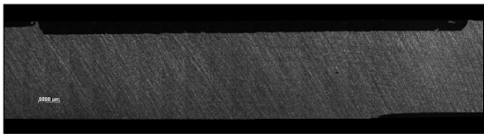
Fig. 7. Cross-section of specimen welded by tool 3 at a feed rate of 125 mm/min.
