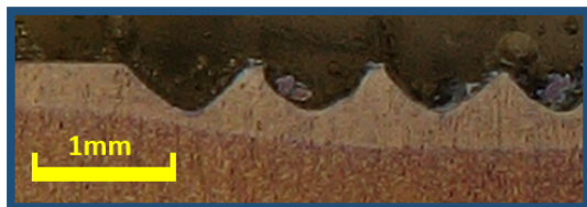
Fig. 3. Effect of surface heat treatment with a specific heat input of 150 Ws/mm on specimen 22.
