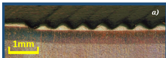
Fig. 5. Vicinity of the machined peak after surface treatment. a) specimen 22 b) specimen 24.
