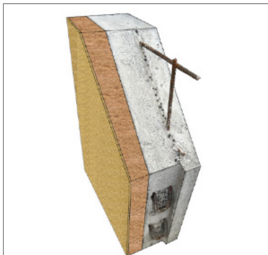
Fig. 2. Liapor wall structure with cellulose insulation
