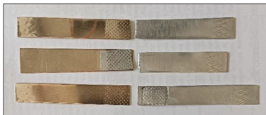
Fig. 4. Samples welded at higher pressure.
