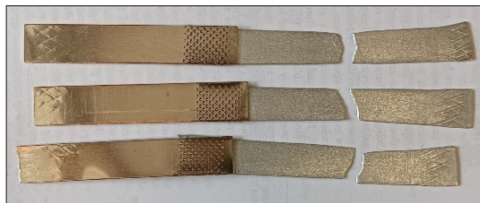
Fig. 3. Samples welded at lower pressure.
