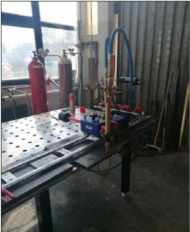
Fig. 1. Flame-cutting equipment used for preparing the test specimens.
