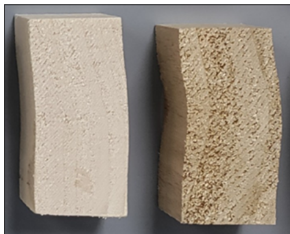
Fig. 16. Typical fracture pattern of the test specimens – LT90.
