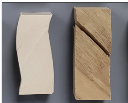
Fig. 13. Typical fracture pattern of the test specimens – LT45.
