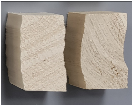
Fig. 19. Typical fracture pattern of the test specimens – RT45.
