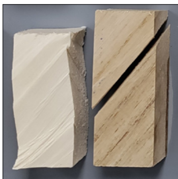
Fig. 7. Typical fracture pattern of the test specimens – LR45
