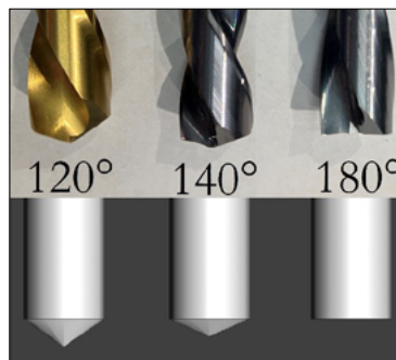
Fig. 6. Vertex angle options for pilot drills and their respective pilot hole geometries.
