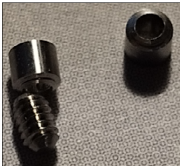
Fig. 4. Screw after failure, two broken-off screw heads and one threaded shaft.
