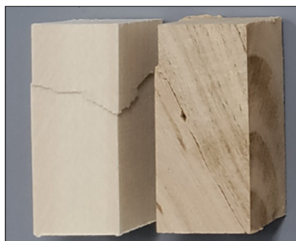
Fig. 4. Typical fracture pattern of the test specimens – LR0.
