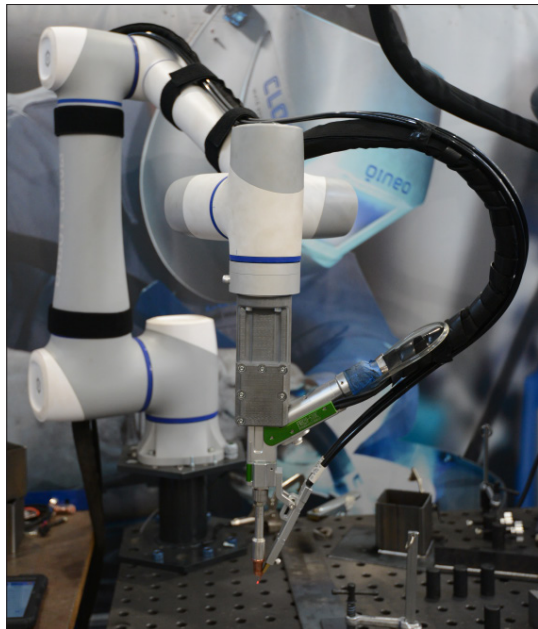
Fig. 7. FWH20-S10A laser welding gun mounted on CR10A Dobot [4]
